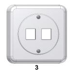
3 Surface mounted (AP) with surface mounting frame 89 x 89 mm, 86 x 86 mm cover frame, and Ø 63 mm front plate, height: 54 mm
